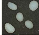
3D printed spherical aggregate
