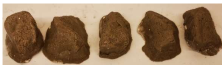
Artificial aggregate made from AAM
