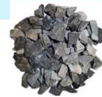
Angular aggregate (cold bonding and crushing)
